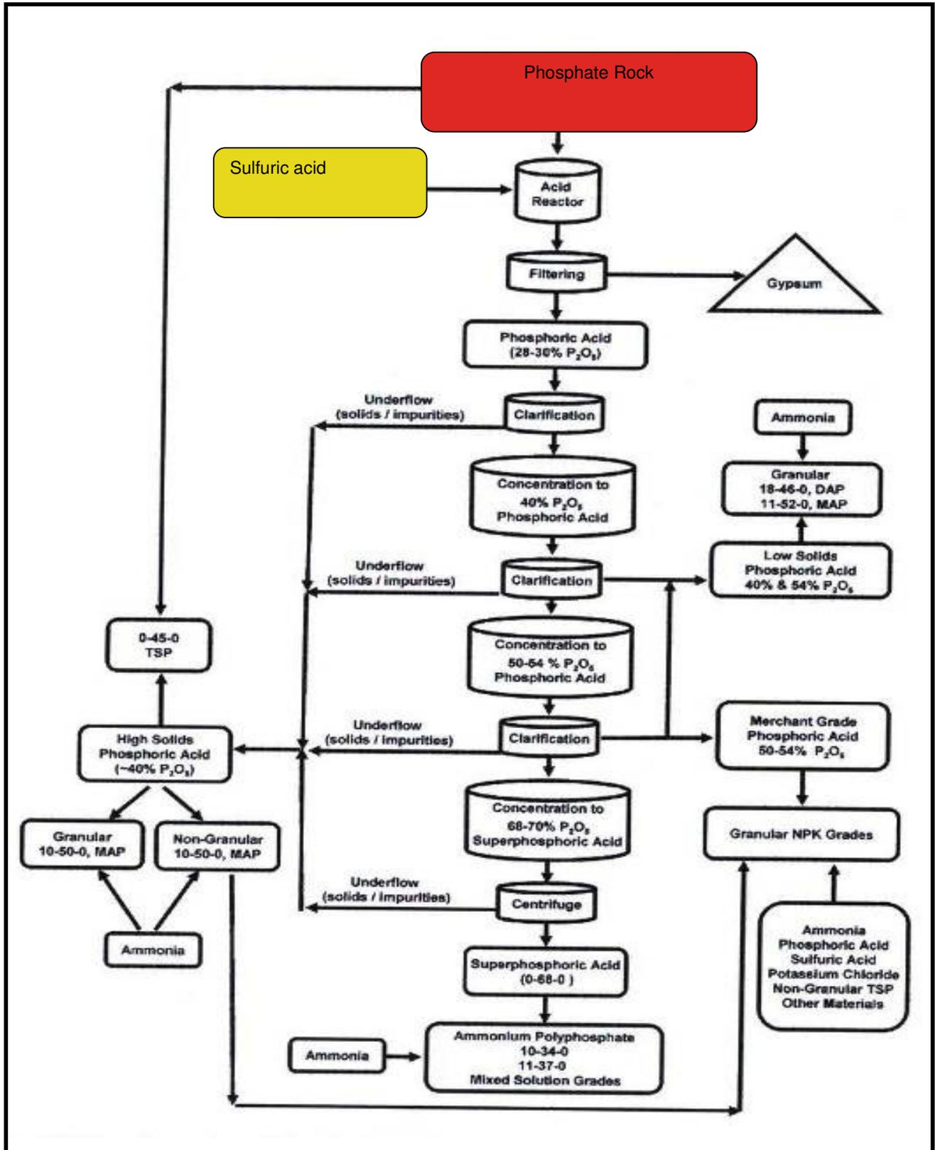
Figure 2: Phosphoric Acid Production Process
